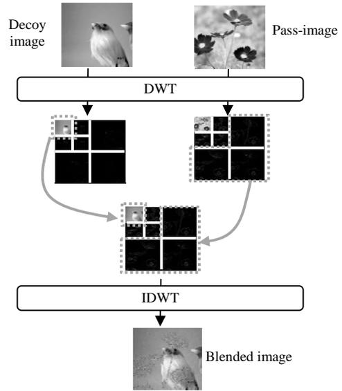
Fig. 2 Overview of the image blending procedure.
